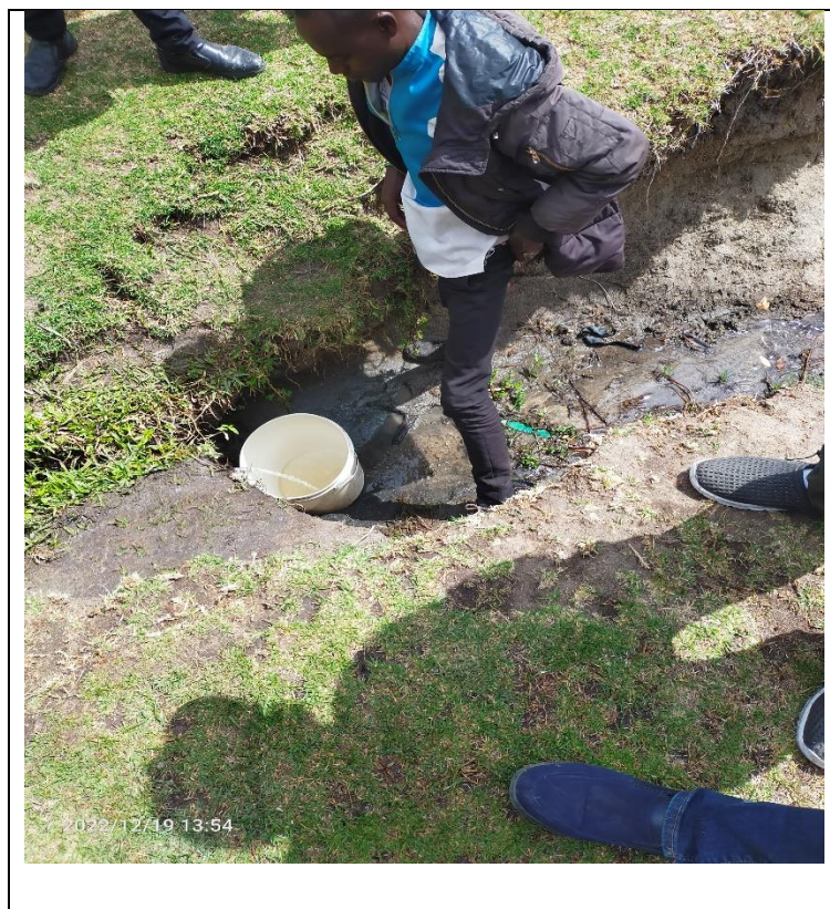
Plate 4: Volumetric method of discharge measurement used at project site
